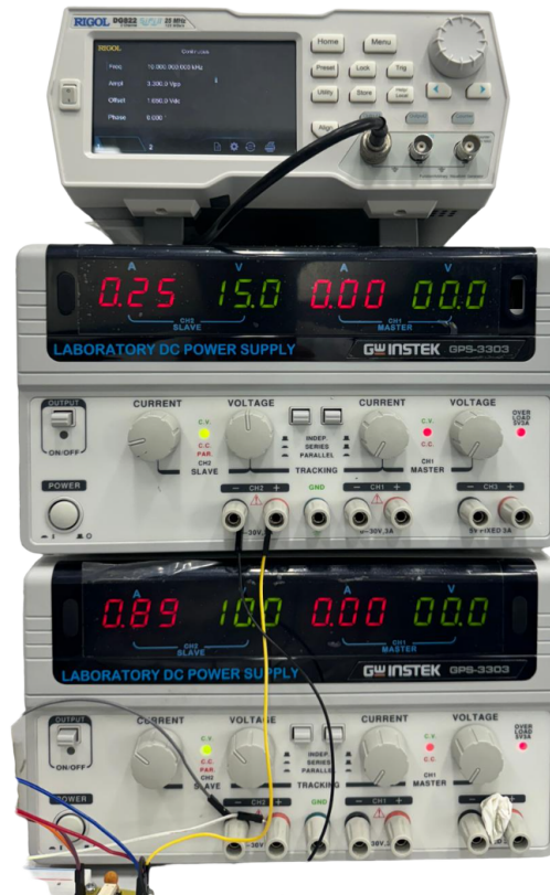
Figure 9: Two power supplies set up, demonstrating the different voltage settings for the Buck circuit and TLP250 as required in the experimental setup.
