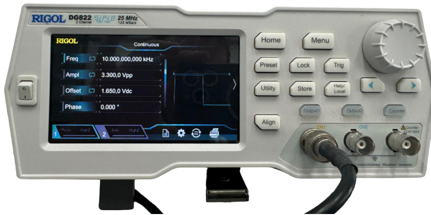
Figure 10: Function generator set to specific parameters, demonstrating the desired settings for controlling the MOSFET in the Buck converter circuit.
