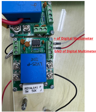
Figure 10: Connecting the voltmeter cables to the circuit for accurate voltage measurements.
