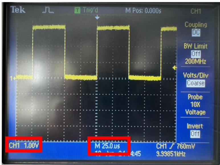
Figure 11: The oscilloscope screen displaying the signal with the attenuation correctly set.
