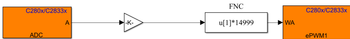
Figure 7: Simulink block diagram for dynamic PWM control via a potentiometer.
