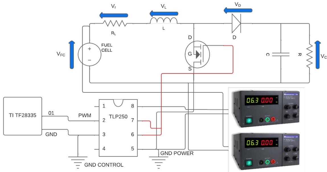
Figure 1: Connecting the TI TF28335 board with the TPL250
