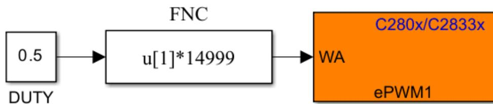
Figure 2: Block diagram of configurations for PWM signal generation.
