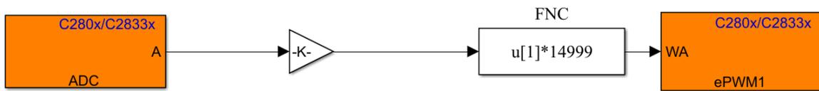
Figure 7: Block diagram in Simulink for dynamic PWM control via a potentiometer.
