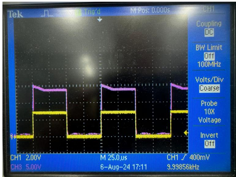
Figure 11: Oscilloscope capture showing the PWM signal. Channel 1 (yellow) represents the signal generated by the TI board, and channel 3 (pink) shows the signal processed by the Gate Drive TLP250.
