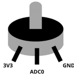
Figure 10: Potentiometer Connection
